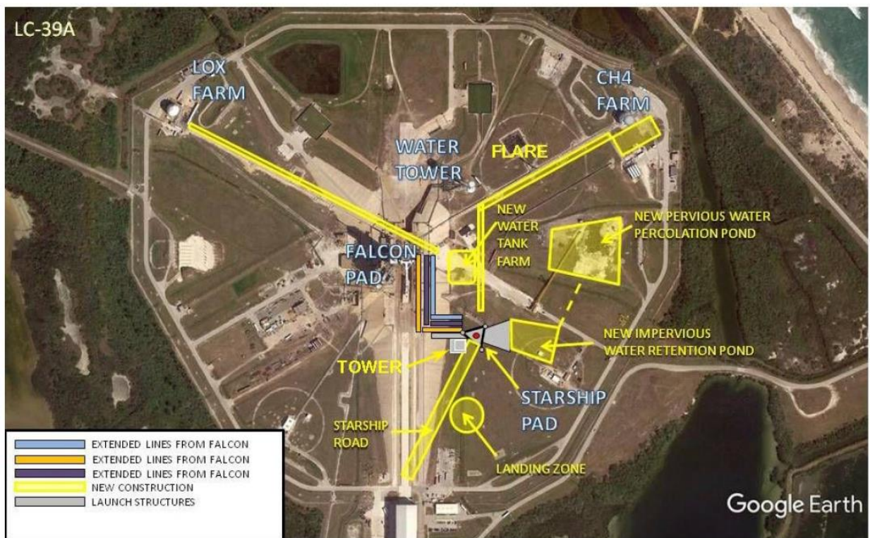
Figure 2-2. Proposed LC-39A Configuration with Starship/Super Heavy Launch Pad and Associated Operational Structures Shared or Separate from Falcon
